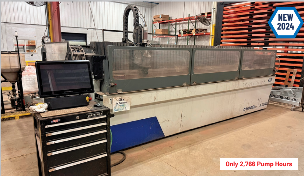
9' x 15' Wardjet Model X-2040 Five-Axis CNC Waterjet w/ 60,000 PSI Intensifier Pump
