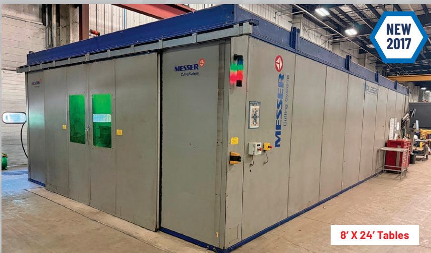
6,000 Watt Messer Model MMXCEL CNC Fiber Laser w/ 8' x 24' Shuttle Tables, Camfil GS8 Dust Collector, Chiller
