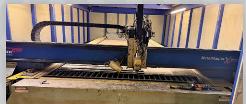
9' x 15' Wardjet Model X-2040 Five-Axis CNC Waterjet w/ 60,000 PSI Intensifier Pump
